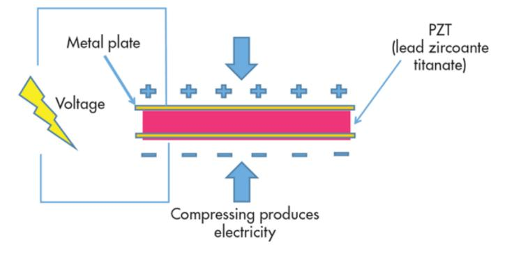
That's it, a simple application of mechanical pressure, the squeezing of a crystal and suddenly you have an electric current. You can also do the opposite, applying an electrical signal to a material as an **inverse piezoelectric effect.** It works like this:
